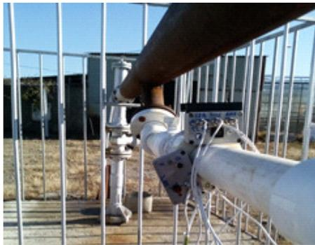
Fig. 2. Exterior of tube supplying geothermal water and device with electronic components installed on it
