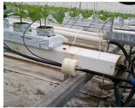
Fig. 3. Acoustic-magnetic device installed in hydroponic solution supply system
